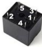
2, 5 - Relay Coil connection 1 - Common 3 - NO 4 - NC
